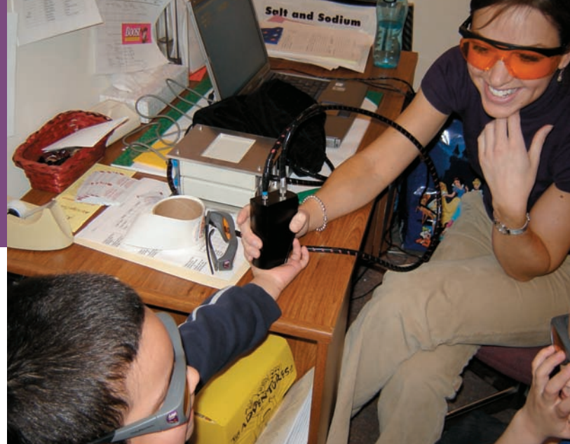
Stephanie Scarmo scans the palm of a preschool child with a portable spectrometer that reads pigment levels known as carotenoids.
